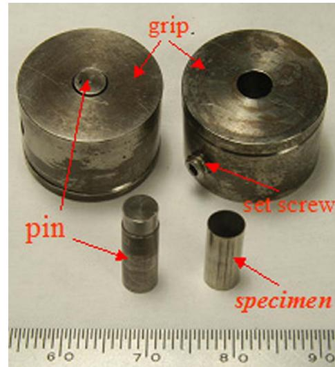
Fig. 4 Photograph of the grip parts and the specimen
